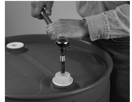
3. Torque insert with drum wrench or 1/2" drive torque wrench and a Colder torque socket tool (Colder PN 2408900).
