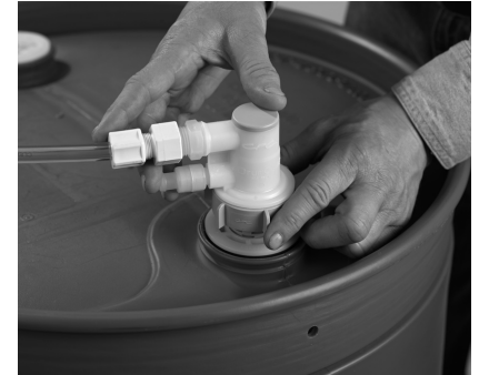
3. Turn the coupler locking ring clockwise until stop is reached (approximately 2 full turns); valve is opened during this process.
