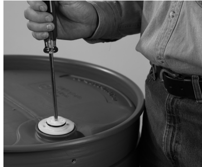
1. Turn shipping plug counterclockwise to remove. (Use a large, flat blade or #4 Phillips screwdriver.)
